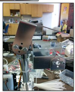
To set the correct servo positions, remove the two servo horns from the servo crowns. Use the joystick to move the servos into the lowest and closed values (the A button and the X button). Replace the servo horns in the closed and down positions and secure them with the servo screw.
