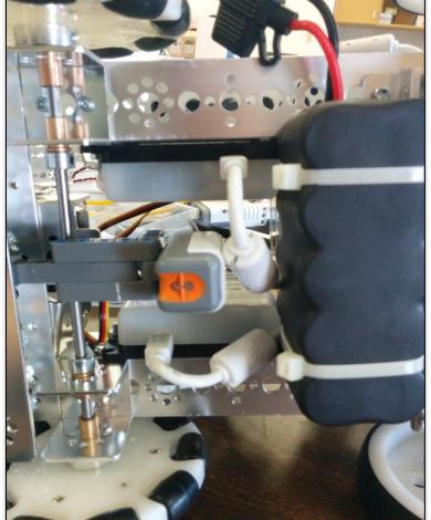
Secure the robot controller to the two 144mm L brackets. I used hook and loop.
