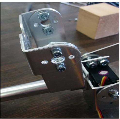
Connect two rounded L brackets to the pivot bracket to complete the gripper.
