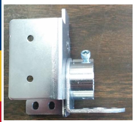
Attach the servo mount to the tube clamp with the rounded L bracket between them.
