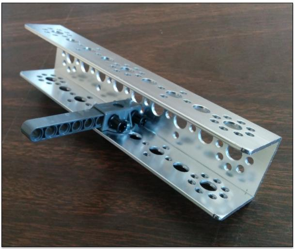
Connect the LEGO® 9 hole straight beam to the hard point connecter with the two pegs.
