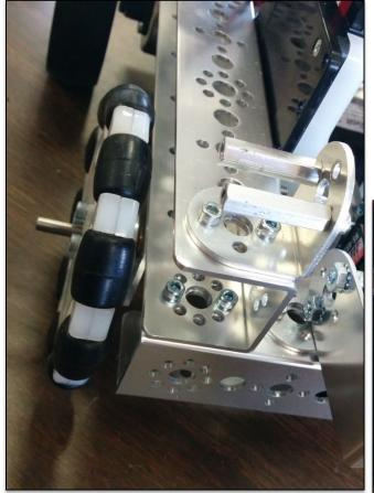
Bolt two stand offs to the rounded L bracket. I used one inch standoffs but two inch standoffs will work as well.
