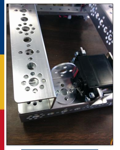
Attach a rounded L bracket to the 166mm C channel next to the servo. This is only used as a mechanical stop so the arm does not swing too far back.
