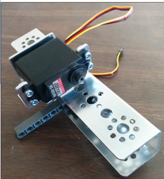
Bolt a servo on to the servo mount.
