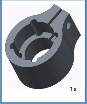
Use four of the shorter Tetrix® screws to attach the tube clamp to the top of the pivot bracket.
