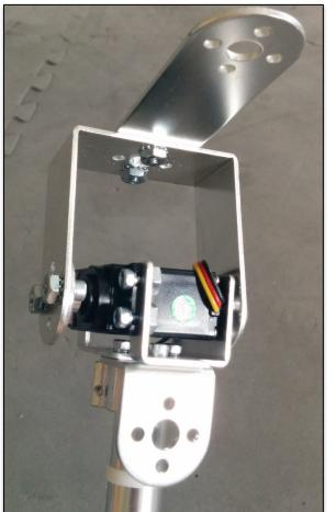
Attach the flat bracket to the pivot bracket.
