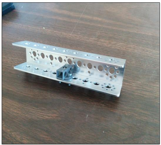
Attach one LEGO® hard point connector to the 166 mm C channel.
