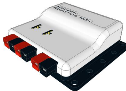
Figure 7 - New Motor Controller has two DC motor channels and uses Anderson Power Pole connectors
