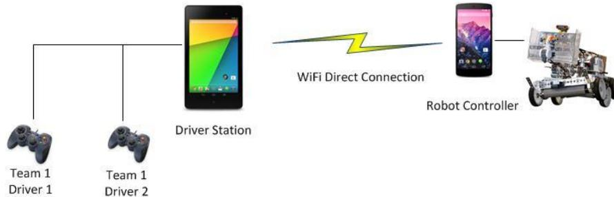
Figure 1 - The new FTC platform is a point-to-point solution.
